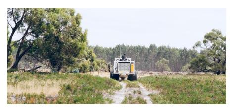
Seismic surveys require a mobile energy source to send sound waves deep into the ground and an array of recording devices planted in the ground in a pattern around the energy source. As the sound waves travel downward, they are partly reflected back to the surface at the boundaries between layers of different rock type.
